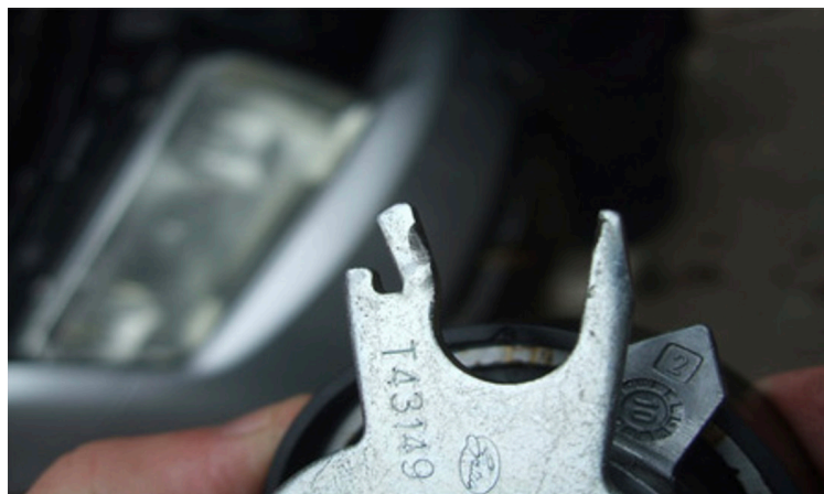
Here we can see unusual wear on the prong
