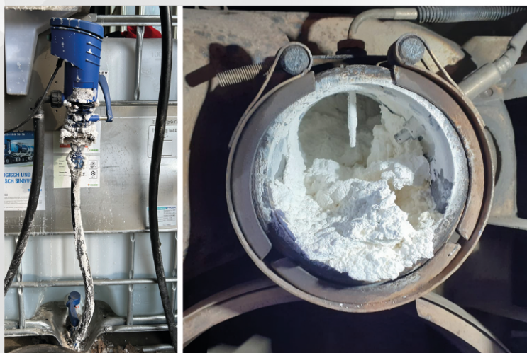
Problems in the AdBlue® system due to deposit formation. SCR system protection: "The additive for the additive".
