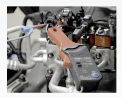
There are many solenoid valves in the heat pump systems. Inspect them in terms of input signals and currents that steer their operation. If necessary, flush or replace.
