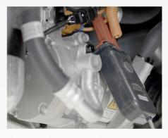
The high-voltage electrical AC compressor requires special lubricant. When troubleshooting, besides visual, sound, and OBD inspection, it is worth including input signals and current diagnostics.
