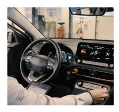
The system performance check belongs to the troubleshooting fundamentals. Take time to thoroughly inspect the output of each of the heating and cooling modes.
