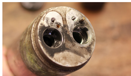
Excessive contamination spotted on the receiver dryer's couplings. This system suffer from severe contamination and must critically be flushed.
