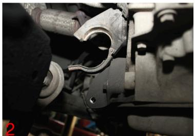
With the engine supported from above, remove one of the gearbox support bracket bolts and lower the gearbox and engine slightly. Unbolt and remove any pipes attached to the gearbox mount (Fig 3).
