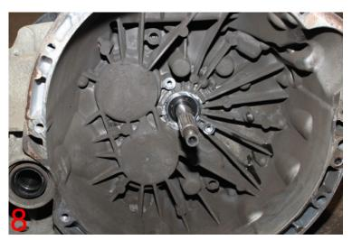
Refit the new CSC, taking care not to compress it prior to fitment. Make sure to use the original or new and correct bolts – don't be tempted to replace them with something 'similar'! Once completed, fit the new extension pipe, making sure the clips locate correctly.
