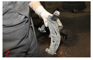
Unclip the concentric slave cylinder (CSC) extension pipe, which may be useful for a future blanking plug. Unbolt and remove the CSC, carefully noting the gearbox seal (Fig 8) condition.
