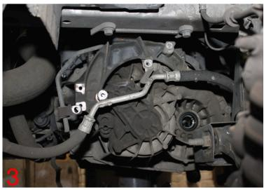
Now remove the mount altogether, and stow and secure the A/C pipes clear of the gearbox. Cut the cable ties, securing the over gearbox harness lid, ready for removal. Unclip and disconnect the gearbox, breather pipe, then remove the two bolts securing the harness box (Fig 4) to the gearbox and remove it to allow access to the bell housing bolts, whilst leaving the harness in-situ.
