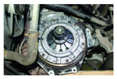
Re-fit the gearbox in reverse order of removal and refill the gearbox with oil. Before fitting the clutch cable, check the cable for free operation and when adjusting always remember to leave a little free play at the top of the pedal to ensure a full release. Once the repair is complete, carry out a road test to ensure the clutch and gear change operation is correct and that all electrical items have been reset after re-connecting the battery.
