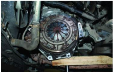
At this point we noticed that the release fork/arm had restricted movement due to the build-up of clutch dust at the pivot points and would not return to its rest position (see below), so we cleaned out the area with clutch and brake dust cleaner, and inspected the release system for any wear and carried out a check for correct and full operation
