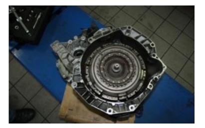
LuK trained and certified technicians can replace the double clutch assembly and engagement mechanism. Release the transport locks and adjust the clutch with the LuK special tools 400 0418 10 and 400 0423 10. Check the DMF anti-back lash ring for damage; our customer requested that we change the dual DMF whist the gearbox was removed.
