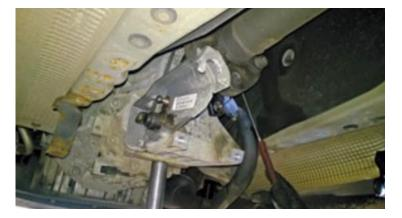
Remove both parts of the gear linkage: part one is achieved by removing the plastic cover from the linkage housing and then removing the cable by releasing the ball joint. Part two of the process is completed by removing the retaining pin from the selector rod above the output flange and disconnecting.
