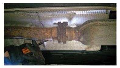
Disconnect the exhaust centre joint by removing the three bolts (these may be corroded) and then remove the exhaust front pipe support bracket. Now remove the rear gearbox mounting, before disconnecting the prop-shaft from the gearbox.
