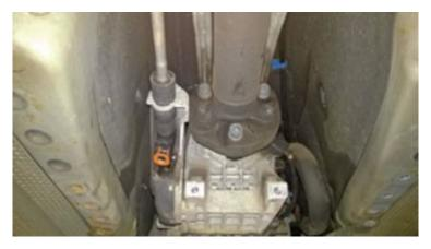
Remove the rubber cushion drive unit, noting the position and colour of the bolts and washers as they have different locations. Now disconnect the hydraulic clutch pipe; the easiest point for this is where the hydraulic pipe comes through the transmission tunnel on the O/S. Once disconnected, the pipe connection needs to be blanked to prevent the fluid leaking out.
