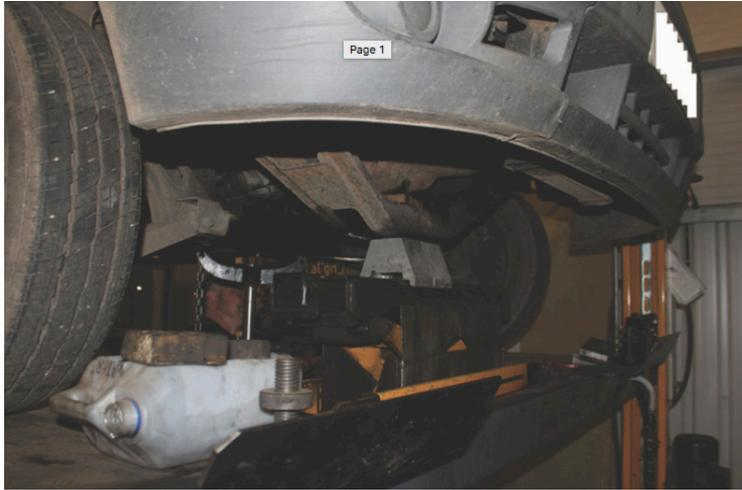
After that, remove the oil feed and return pipes from the steering rack body (see below) and cap to prevent the oil system draining.
