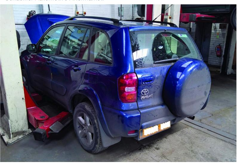
In this article, we are replacing the clutch and Dual Mass Flywheel (DMF) in a Toyota RAV4 2.0 D4D with permanent four-wheel drive, which has covered more than 130,000 miles. The customer reported that the clutch slips under full load, which a quick road test confirmed, and clutch replacement was advised
