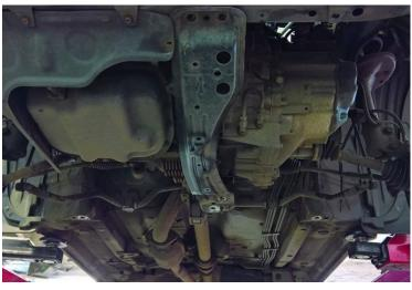
Now drain the oil out of the gearbox and transfer box and, once the oil has drained, remove the O/S/F driveshaft by sliding out of the transfer box and store in a safe and clean area (see below).
