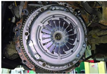
Re-fit the gearbox in reverse order of removal, refill the gearbox and transfer box with the correct quantity and specification of oil and, after connecting the battery, reset all electrical items as required and carry out a road test to ensure the repair is complete.
