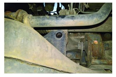
Support the front sub-frame with a transmission jack and remove the sub- frame retaining bolts, lower the transmission jack and remove the front sub-frame (see below) and then remove the gearbox cross member/cradle.
