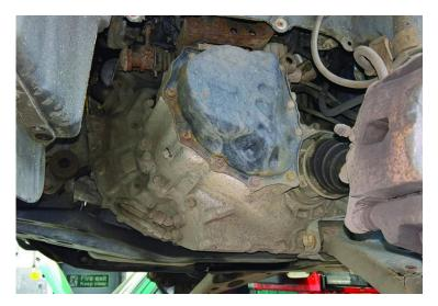
Raise the vehicle. Now we need to remove the front sub-frame, so disconnect the anti- roll bar clamps, remove the front gear-box mounting, disconnect both bottom ball joints, and take out the two bolts that hold the steering rack to the front sub-frame (see below) and secure the steering rack to the engine bay to hold in place.
