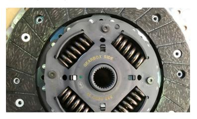
Mount the clutch assembly onto the flywheel (see below), before inserting, tightening and torquing all clutch bolts evenly and sequentially. Once torqued, remove the clutch alignment tool.
