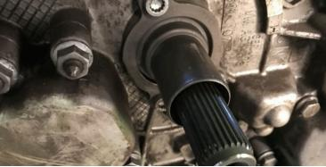
Fit the release arm and bearing. If plastic/nylon runs on metal, no lubrication is required; if metal runs on metal, lubrication is required and a light smear of high melting point grease is best practice.
