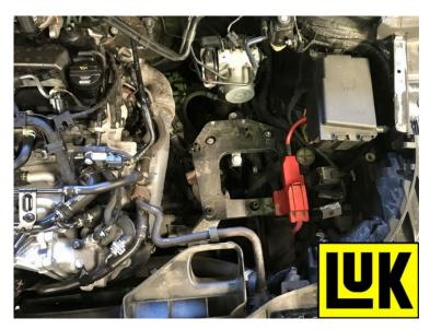
Disconnect the gear change cables, and remove the clutch slave cylinder, leaving the hydraulic pipe connected. Detach the starter motor cable and unscrew the top starter motor bolt, before disconnecting the reverse light switch multiplug and removing the top bell housing bolts.
