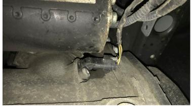
Next, detach the lower bell housing bolts, leaving two easily accessible bolts to support the gearbox, before removing the bottom pendulum gearbox mount. Alistair used two transmission jacks to support the engine and gearbox respectively, before using a ladder to gain access to the engine bay and remove the gearbox mounting bolts.
