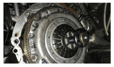
Before refitting the gearbox, ensure all wiring etc. is clear of the bell housing area, so as not to get trapped, while also checking the gearbox alignment dowels are fitted to the engine and that the release mechanism in the gearbox is fitted and functioning correctly.
