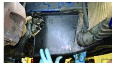
Support the engine, then remove the engine mount and disconnect the mounting bracket from the engine block. This cannot be removed as there is not enough clearance, but can be manoeuvred to allow belt replacement. Now remove the upper timing belt cover, and then with access through the O/S/F wheel arch, take off the two lower timing belt covers, rotate the engine in a clockwise direction and align the timing marks. Then insert locking tools into the crankshaft, and the camshaft.
