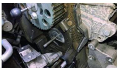
Now take out the water pump by removing the three retaining bolts and easing the pump out of the engine block, and then drain the engine coolant into a tray placed under the vehicle. Once drained, ensure the mounting and sealing faces for the pump are clean and dry, install the new water pump and tighten to the manufacturer's specification. Remove and dry any remaining coolant in the timing belt area and fit the new idler and tensioner.
