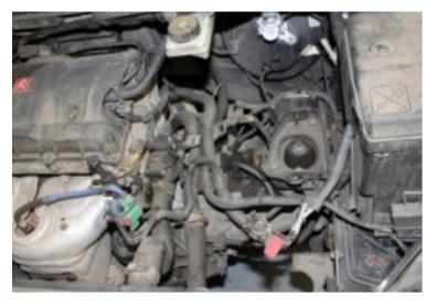
Release the gear linkage from the gearbox (you can also remove the gear change pivot weight to aid removal). Whilst in this area, there are two bolts that can be removed – one for the starter motor and one for the gear linkage bracket on the outside of the bell housing.
