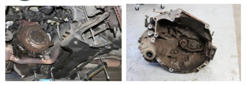
On the gearbox, remove the release bearing and then inspect each of the sleeve/guide tube, release fork and ball pivot for wear and replace if required. Remove any clutch dust by cleaning the bell housing and fit the new release bearing. Lightly lubricate the clutch splines on the input shaft with high melting point grease and evenly distribute by fitting and sliding the new clutch plate to the input shaft and wipe off any excess. This also confirms that you have the correct clutch plate.
