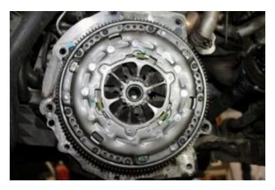
Clean the bell housing of the gearbox, replace the release bearing and ensure that there is no wear to the clutch release fork and gearbox snout. Then lubricate the pivot points that are metal-to-metal with a smear of high melting point grease. Ensure the dowels are located properly on the engine and that the sandwich plate is positioned correctly.
