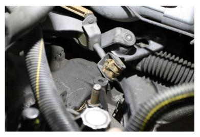
Make sure the gear link arm is stowed securely out of the way. Install the engine support beam before removing the top gearbox mount and also the bracket from the gearbox.
