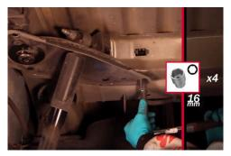
On the left hand side, use a hand-held compressor to compress the coil spring, in order to remove it from the vehicle. Remove the bolts on the mounting plate above the shock absorber.
