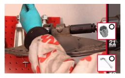
Remove the mounting plate from the shock absorber.
