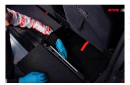
Remove the spare tyre. For the Peugeot 5008, you can find the special access tool just below the lip of the boot wall.
