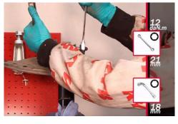
Attach the mounting plate to the top of the new shock absorber.
