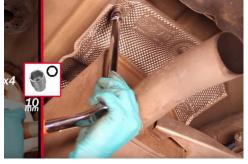
On the right hand side, remove the heat shield above the exhaust, to give access to the coil spring. Use a compressor to remove the coil spring.
