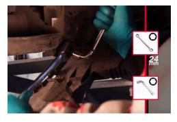
Remove the bottom bolt, then remove the shock absorber and mounting plate.
