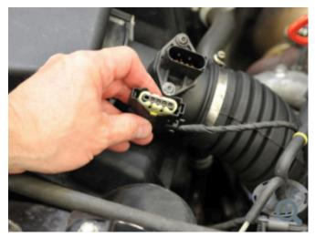
There are many different variants of the hot film air-mass sensor in the newest generations. Depending on the requirements of the manufacturer, they are available with a different number of pins, with or without intake air temperature sensor and with analog or digital signal output.
