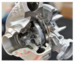
entire exhaust gas energy is used and the flow cross-section of the turbine can be set optimally for every operating point so that, compared with the bypass control, the efficiency of the turbocharger is improved and therefore that of the engine. The ongoing
