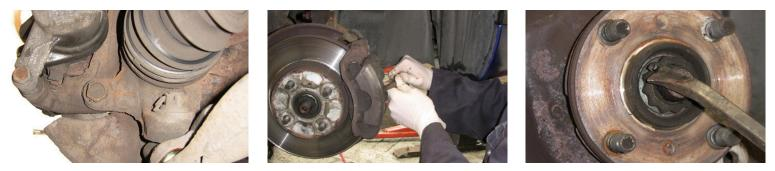
Push the brake cylinder back (see pic, below) and slide the calliper off.
