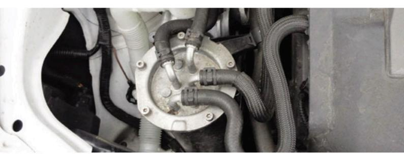
It's been identified that fuel leakage from some VAG vehicle diesel filter housings may occur subsequent to fuel filter element replacement.
