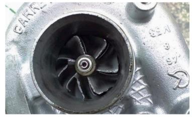
Firstly, look at the inlet compressor by removing the inlet pipe. Spin the shaft and feel for excessive shake or roughness. Hold the centre of the shaft and move it up and down to check for radial wear and push and pull for axial end float – some play is normal. This is the oil clearance that allows the shaft to float on a film of oil.
