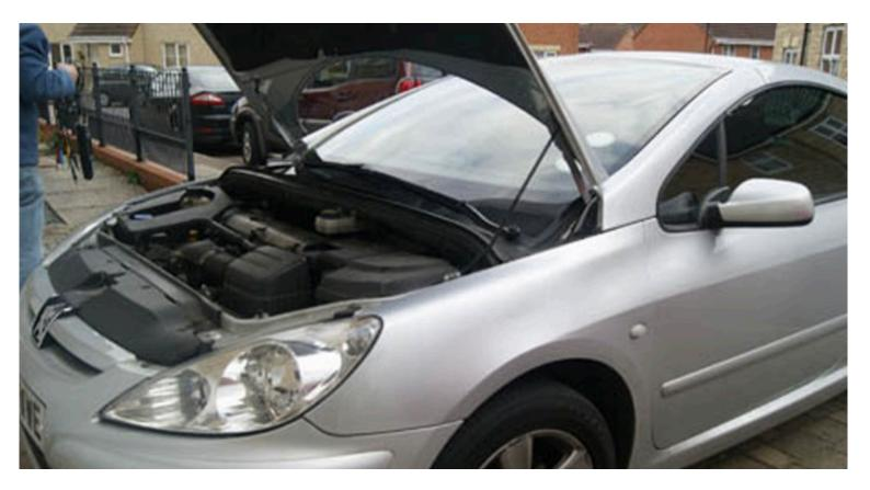
This vehicle came to me on the back of a customer recommendation and had a problem that proved to be anything but simple to resolve. The engine would start first time but any attempt to apply throttle was getting no response unless pumped or pushed to the floor. Once we acquired the right amount of fuel for a reasonable road/fuel pressure test, I noticed that the car ran extremely well at all constant speeds but the problem occurred in stop-start situations. With all this in mind I ruled
