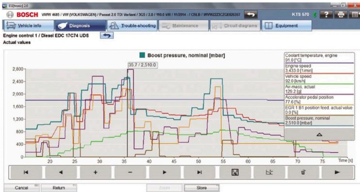
The technician now has the option to play back the capture in a sequence or scroll through the data screen-by-screen and then zoom into millisecond detail if needed.
