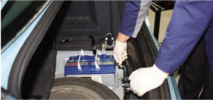
**5. Ensure the battery is correctly located**, in the tray and clamped into position. battery.
